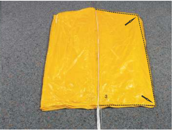
8. Arrange panel 3 (Ultra Cross 100/125). Ultra Cross 75: not applicable Ultra Cross 150: panels 4,3, Ultra Cross 210: panels 5,4,3
