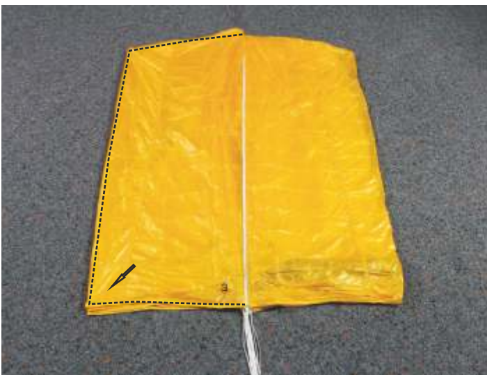
17. Arrange panel 3 (Ultra Cross 100/125). Ultra Cross 75: not applicable Ultra Cross 150: panels 4+3, Ultra Cross 210: panels 5+4+3
