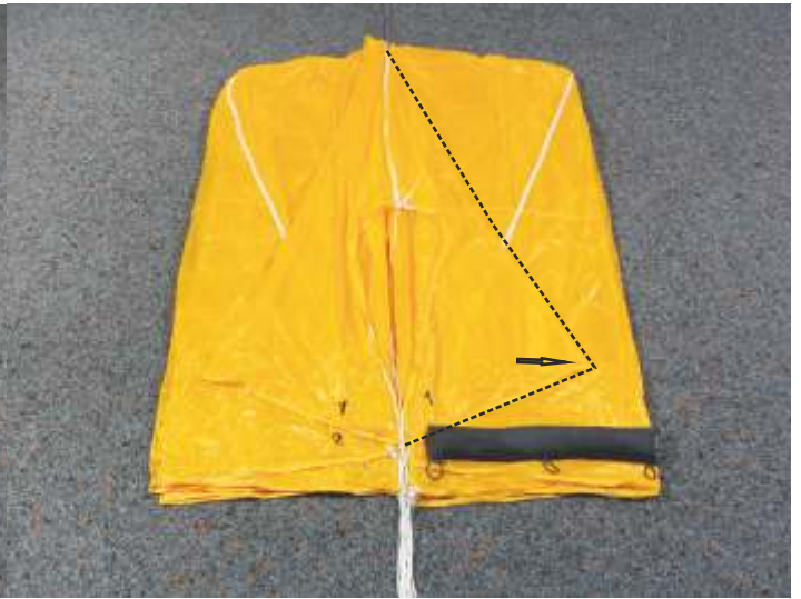
10. Arrange panel 1 (corner panel) and place a packing weight on the hem.
