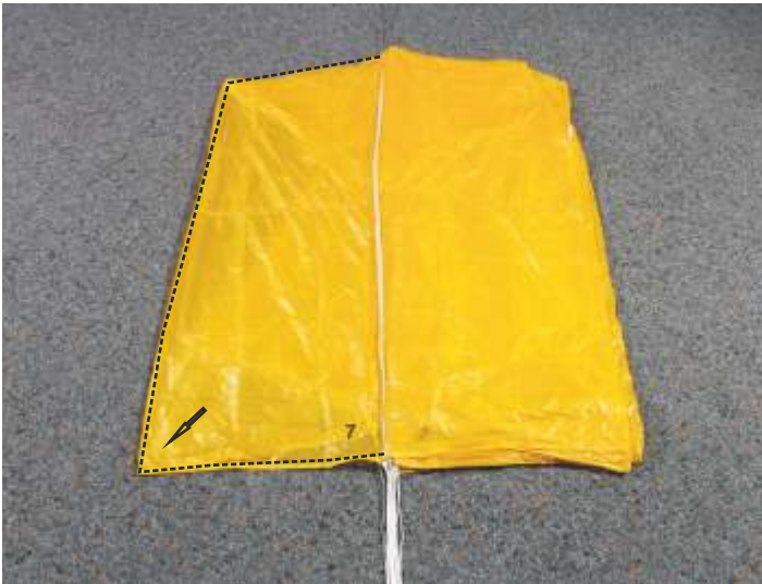
13. Arrange panel 7 (Ultra Cross 100/125). Ultra Cross 75: panel 5, Ultra Cross 150: panel 9, Ultra Cross 210: panel 11
