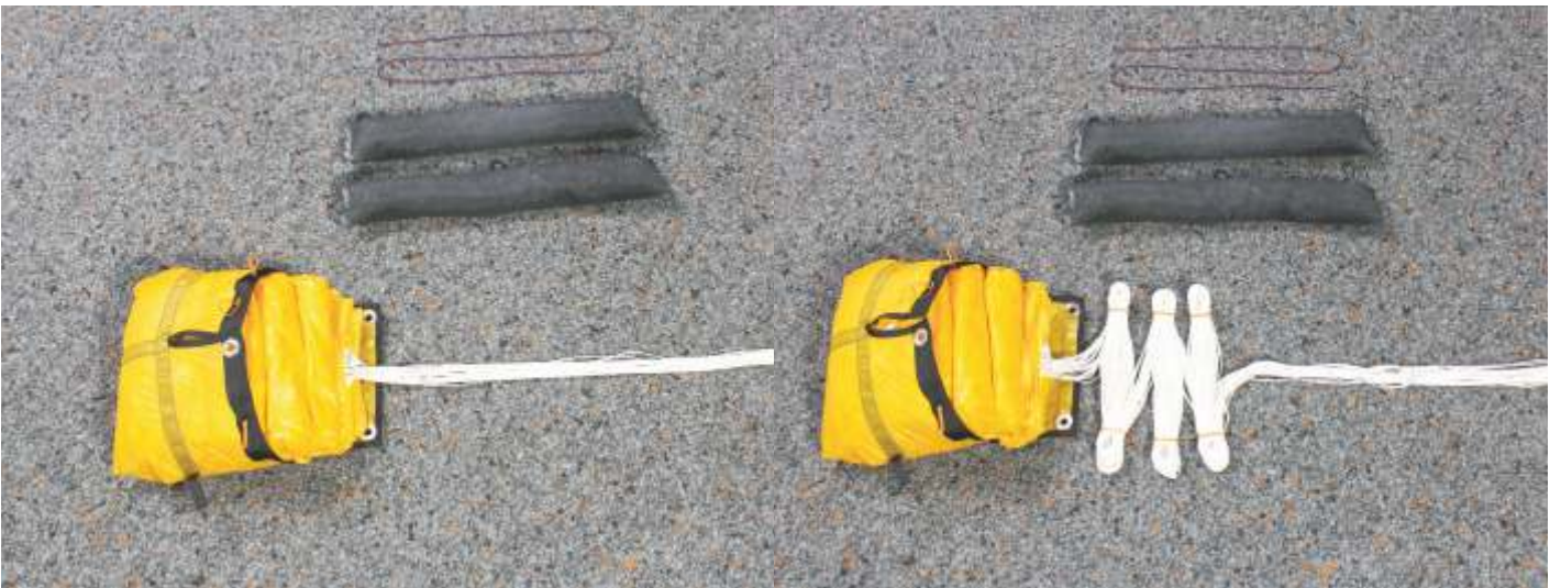
26. Put the S-folded canopy in the deployment bag.
