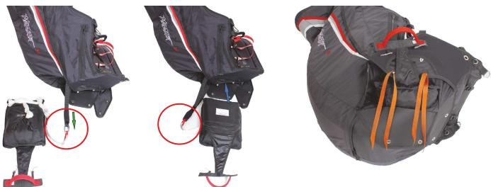
1. Connect the rescue bridle with the harness bridle by looping the bridles or with a quick link (strength > 2400 daN) and fix the connection to prevent slipping (for example by a neopren sleeve).
