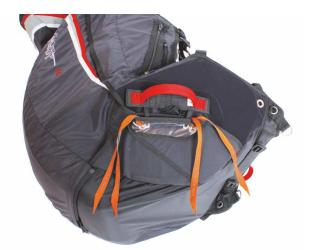
5. Close third container flap with packing cords. Put the pins through the loops.
