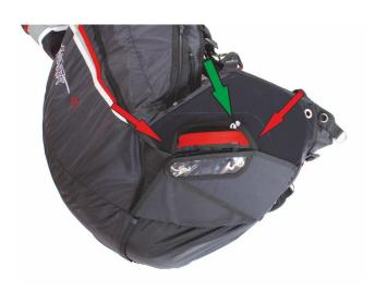
6. Remove all packing cords! Close pin covers and place the handle in the neoprene pockets (red arrow), secure handle with a 2 daN seal threat (green arrow).
