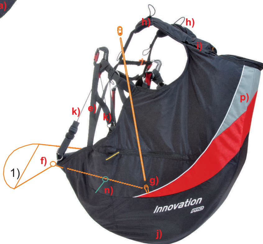
1) Schematic description of how to mount the speedbar (Components partly covered)
